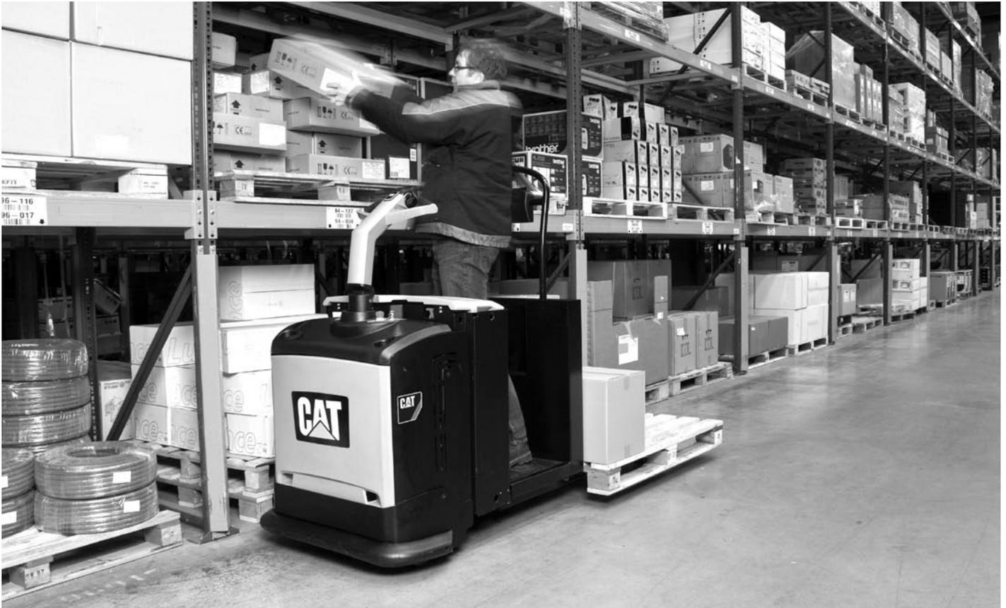
The NQ20NT low-level order picker is designed for fast and safe handling of orders from the picking face to despatch.
